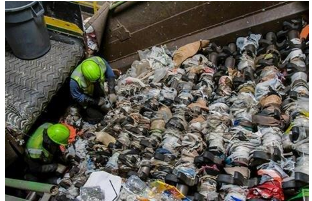
"Tanglers" like plastic bags and film can damage equipment and take time to safely remove.
